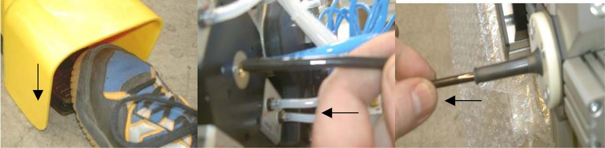
Step 4: Is the cable on the correct position, stop pressing footswith and the module are opening
