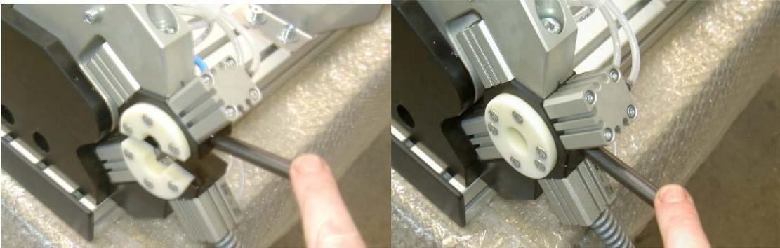
Step 2: Put the grommet in the module
