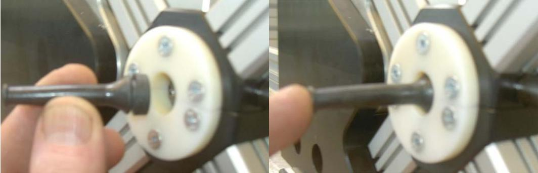
Step 3: Press footswith and push the cable through the module and the grommet
